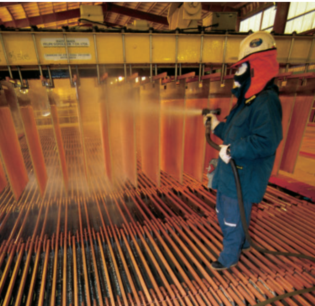
The tankhouse at Escondida, Chile, where several thousand tonnes of 99.999 per cent purity copper cathode are produced every week.
