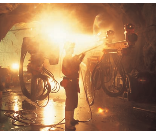
Above: Pressure cleaning drills in a maintenance bay at Palabora's underground mine in South Africa.
