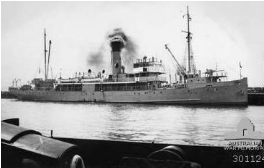
Figure 16: The HMAS Orara at Williamstown. Most of her after deckhouse has been removed and replaced with a winch and minesweeping gear (naval historical collection).
