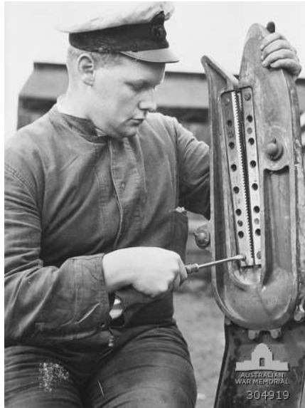
Figure 13: A member of the crew of the auxiliary minesweeper HMAS Goorangai, adjusts the serrated edge of the sweep gear. This apparatus would sever the moorings of the mines (Australian War Memorial naval historical collection).
