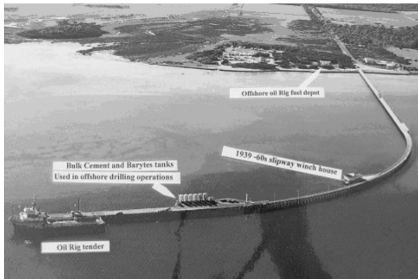
Figure 41: The Long Jetty in the mid-1980s, when it was instrumental to the development of the Bass Straight gas fields. Note the slipway had been removed by this time (Photo: John Woolley collection).
