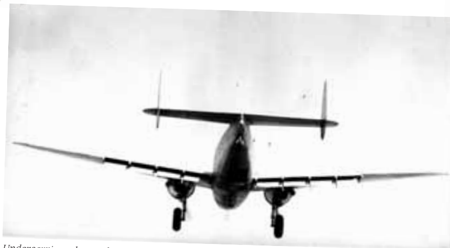
Undercarriage down, the Lockheed prepares to land. Note the extended wing flaps.
