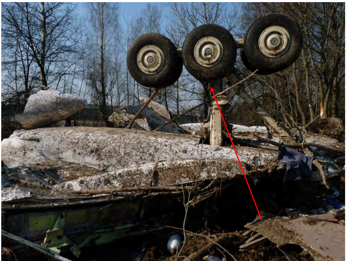
Fig. 13. The left main landing gear in the extended position
