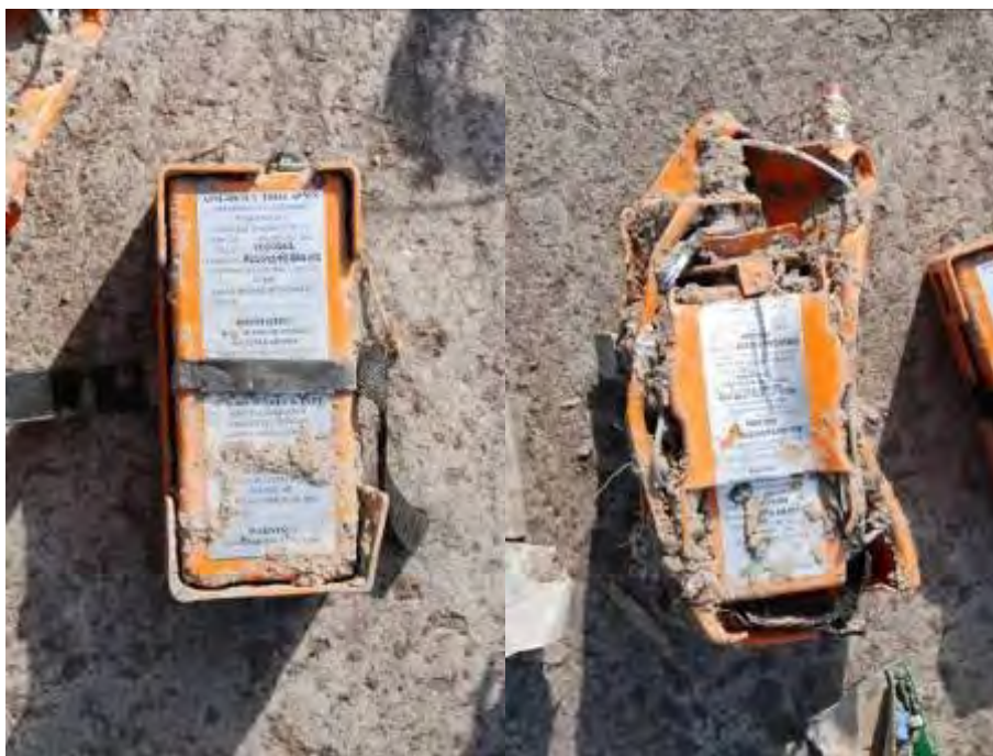
Fig. 36. Emergency radio stations ARM-406AC1 (left) and ARM-406P (right)
