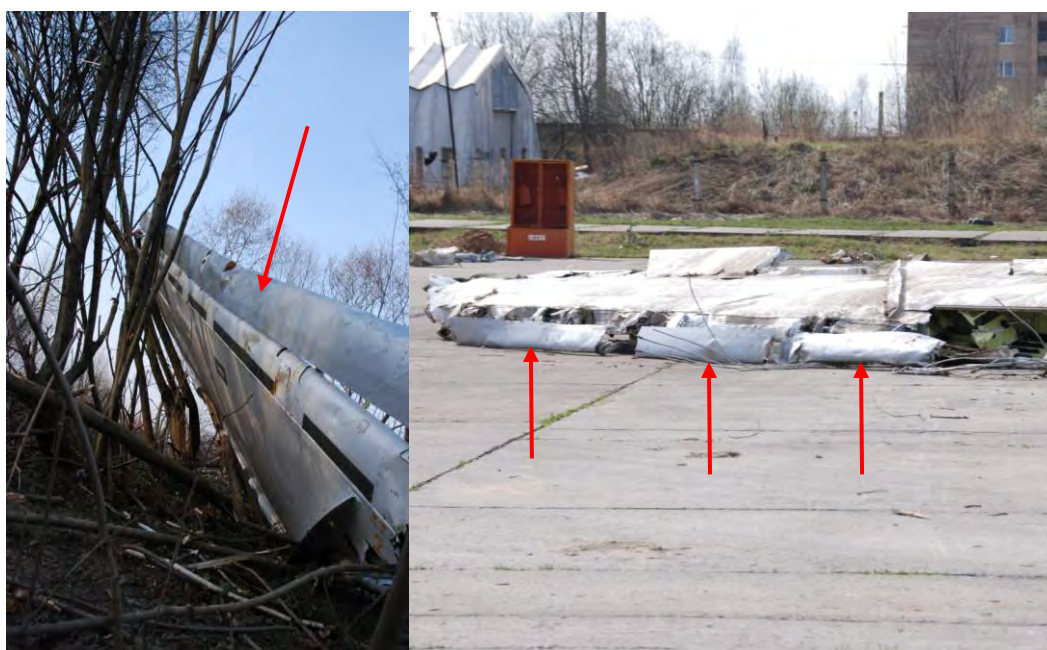
Fig. 7. The slats of the left and right wing of the aircraft in the extended position
