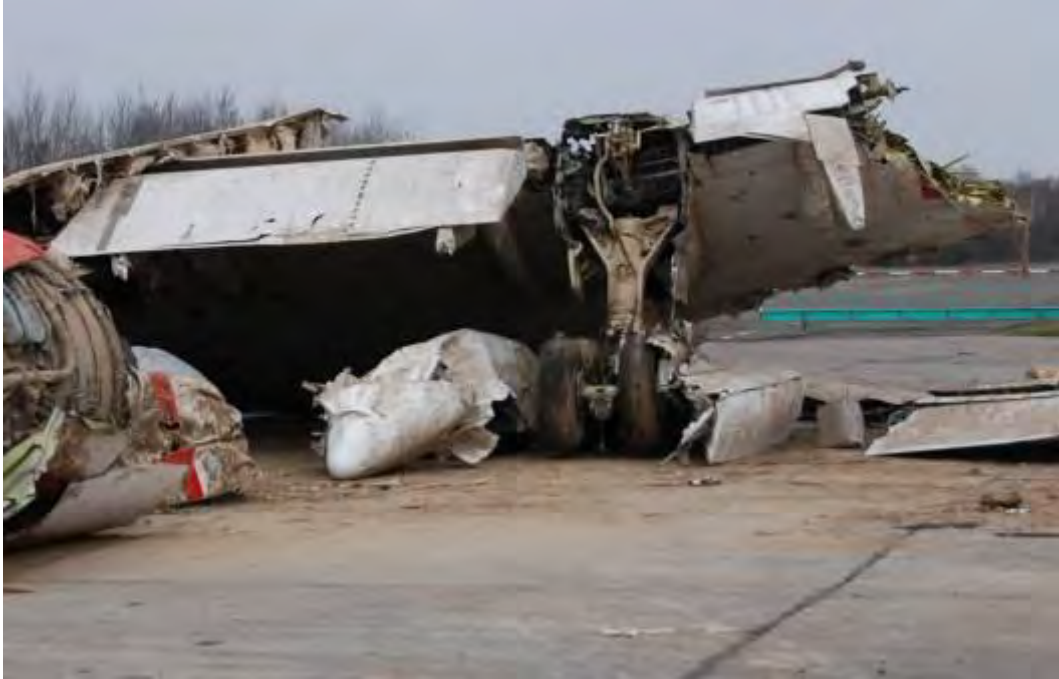
Fig. 15. The trailing edge of the right wing and the right main landing gear
