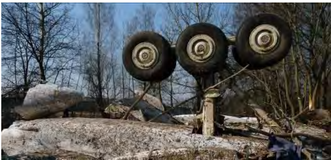
Fig. 28 The left main landing gear
