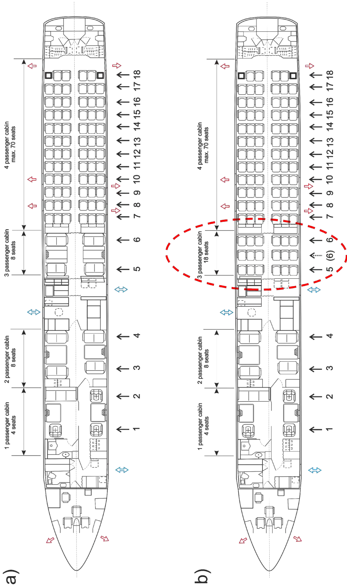
Fig. 2. Plan of the passenger compartment of the aircraft Tu-154M tail number 101 (90A837):
