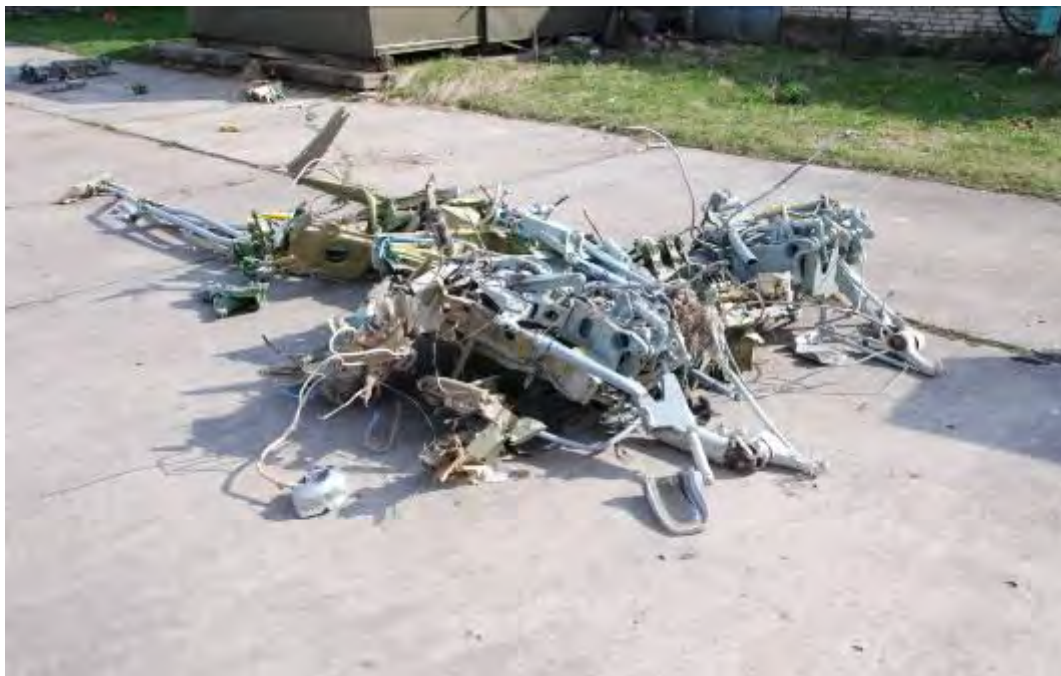
Fig. 26. The remains of the aircraft's controls - the elements installed in the cockpit and under the cockpit deck.
