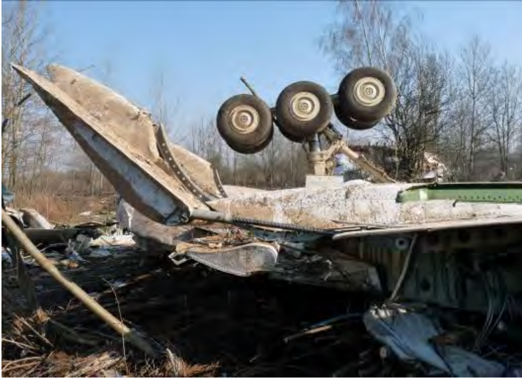
Fig. 29 The right main landing gear
