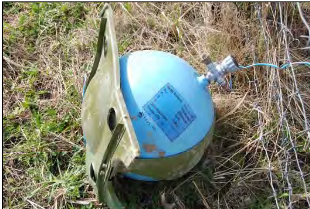
Fig. 32. УБШ-25/150М bottle with a part of its mount and oxygen lines
