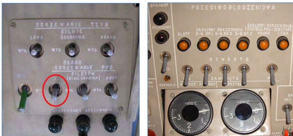
Fig. 22. PPD heating system switching and checking panel (left) and anti-icing system control panel (right) of the Tu-154M aircraft
