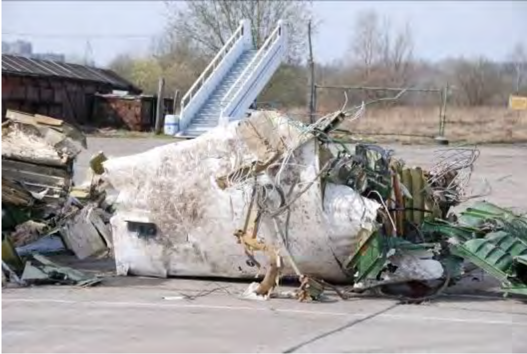
Fig. 8. A fuselage fragment at the fixing point of the nose gear strut
