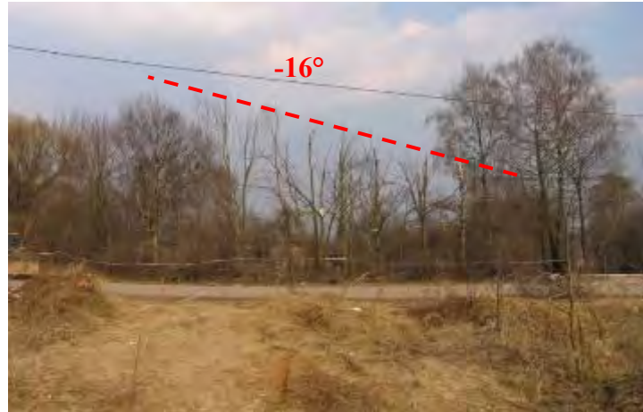
Fig. 8. Trees damaged (item 6 fig. 2) by wings and fuselage with roll of approx. -16° (left)
