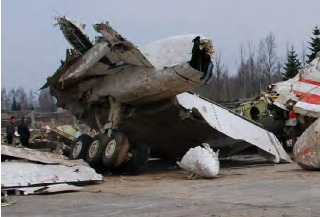
Fig. 17. The trailing edge of the left wing and the left main landing gear
