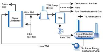
Flash Tanks produce a drop in pressure that causes the methane to vaporize ("flash") from the glycol stream.
