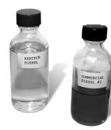
Zero sulfur; zero aromatics, high cetane diesel fuel made by Rentech, Inc., a small fuel development company based in Denver; Colorado.
