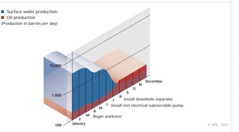
Currently being tested in pilot-scale projects throughout the world, downhole separation may someday deliver significant cost savings and environmental benefits in settings where the technology is applicable. In one recent demonstration (illustrated here), downhole separation decreased surface water production by 95 percent and increased oil production by 50 percent, resulting in a 4-month payback period.
