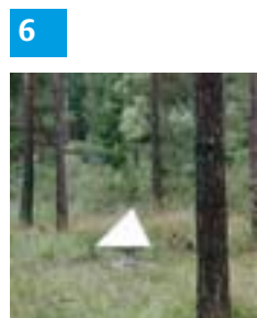
6 One of the 70cm corner reflectors placed under the forest canopy.
