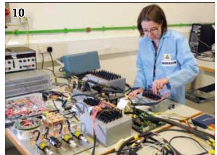
Photo 6 – Computer generated image of LM Photo 7 – Graphic of operational application Photo 8 – Test firing of PAAMS/Sea Viper from Longbow trial platform Photo 9 and 10 – Prototype Fire Shadow actuation electronics and motors and integration 'flat bench' rig with prototype representations of the munition subsystems
