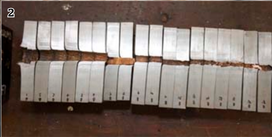
Photo 1 and 2 – Steel target plates with hole from Shaped Charge Attack
