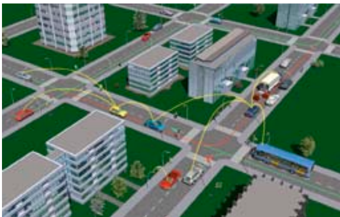
A graphical depiction of a VANET. The unloading vehicle blocks a route and the surrounding vehicles can adopt alternate routes to avoid disruption. Image © Car 2 Car Communications Consortium (used with permission).
