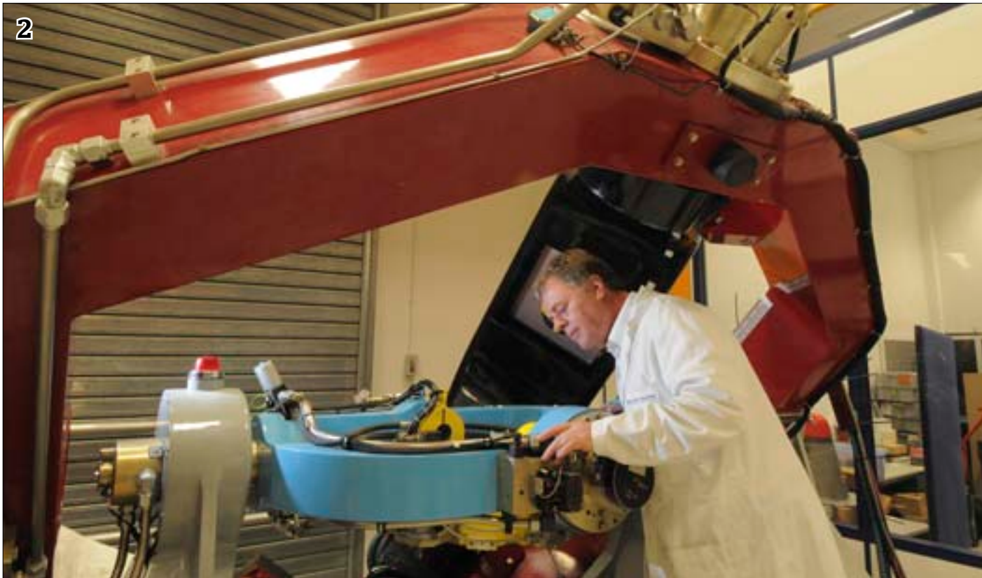
Photo 1 – Mark Slater Photo 2 – System Integration using high performance HWIL flight table Photo 3 – Early integration of the Fire Shadow munition fuselage at the inert build facility
