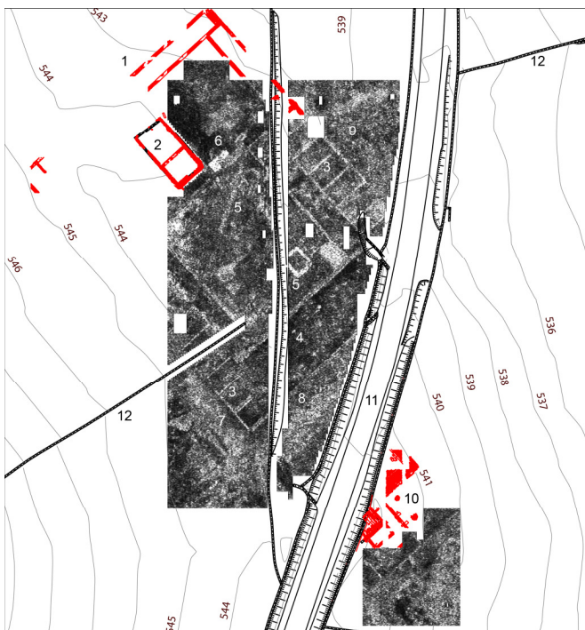
Fig. 4 - Horizontal slice (representing an depth of ca. 70 cm below the surface) of the GPR-survey of the forum area (Map by Verdonck Lieven).
