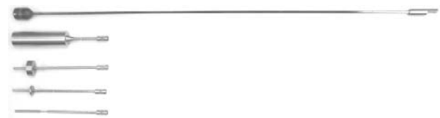
Fig. 4 Comparison of a custom made spindle and four standard spindles
