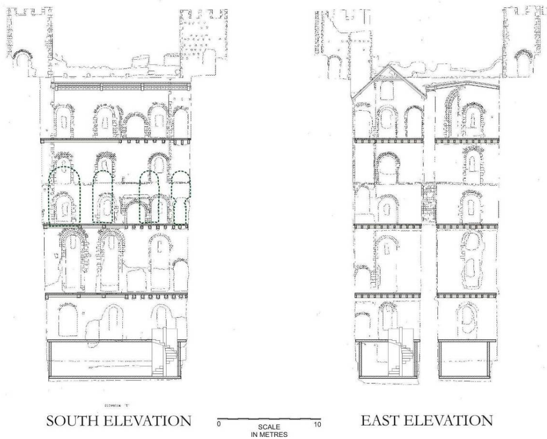
Fig. 7: Possible sections of a re-roofed and floored keep
