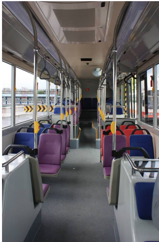
The new MAN bus features a full low floor for the convenience of passenger movement within the bus.
