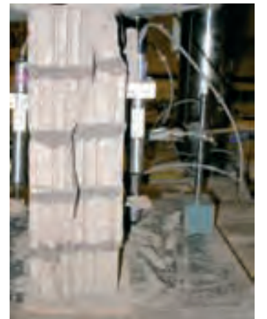
Below left Home using unfired brick internally. Below middle and right Walls were tested to failure in different modes.
