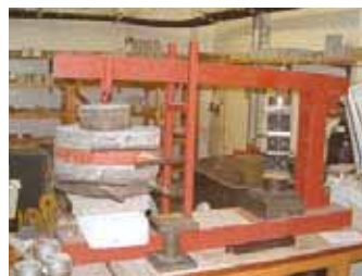
Bitublocks use materials that would otherwise end up in landfill. Opposite shows sample bitublocks being tested in the lab to ensure they can take the loads required for building materials.
