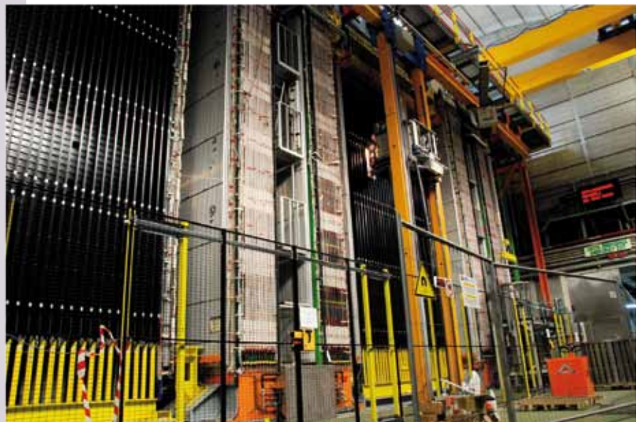
Fig. 10 The OPERA detector in the LNGS underground Hall C.
