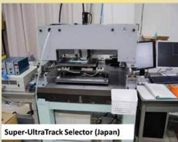
Fig. 12 Two of the many automatic microscopes used for the analysis of the OPERA emulsion films. Top: the system developed in Europe; bottom: the device used by the Japanese groups.
