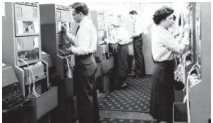
The global communications system, basically a radio system, was the first integrated comm system to span the world. Construction began in 1951. Pictured here is one of the system’s torn-tape relay centers.
