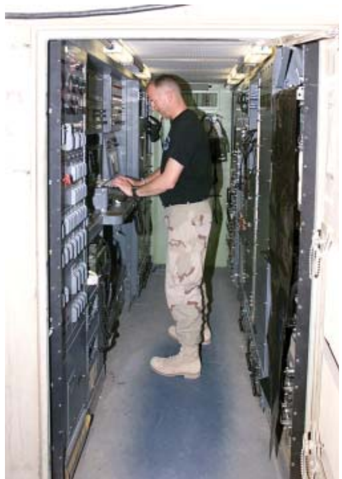
Staff Sgt. Doug Toews programs a secure telephone circuit into the AN/TTC-39A.
