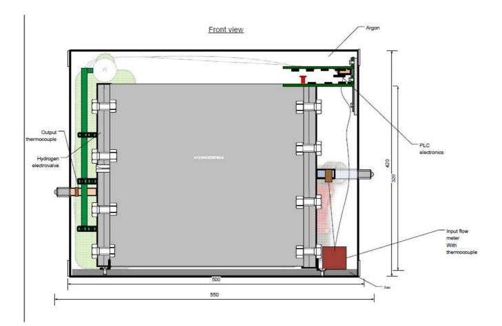
Hyperion schematic internal architecture (multi-reactor model)
