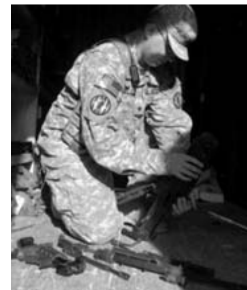
➤ Spec. Zachary Howard frees the legs of the bipod on the 249 squad automatic weapon machine gun to begin the reassembly process.
