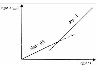
Fig. 9 — Variation of rms jitter with measurement time interval in log-log scale
