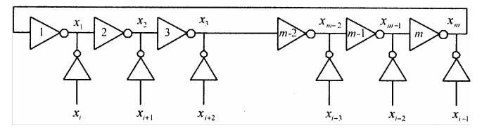
Fig. 3 — Multi-feedback ring oscillator based on single ended delay stages
