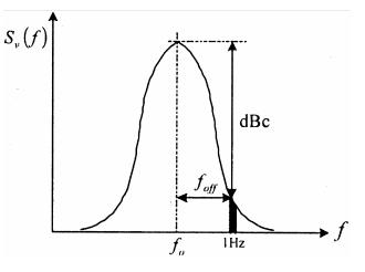
Fig. 7 — Illustration of phase noise per unit bandwidth
