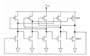
Fig. 2 — Five stages negative skewed delay ring oscillator
