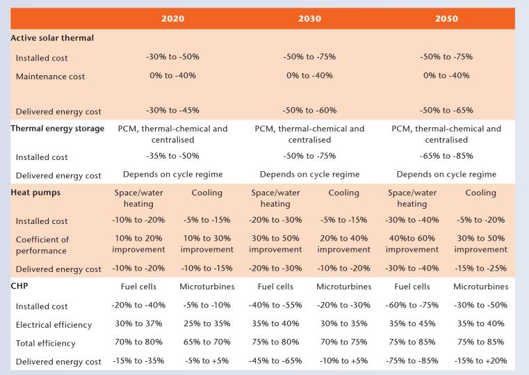
Note: Improvements in costs or performance are expressed as a percentage relative to the base year (2010) specification. However, the electrical and total efficiencies for CHP are actual percentages, not improvements. For fuel cells, the delivered energy cost is for thermal energy and is based on a long-run cost of CO<sub>2</sub>-free hydrogen of between USD 15/GJ and USD 25/GJ in 2050.
