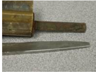
Proper End of Key Tool
