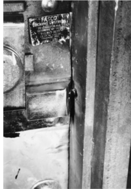
Cut through Bolt
