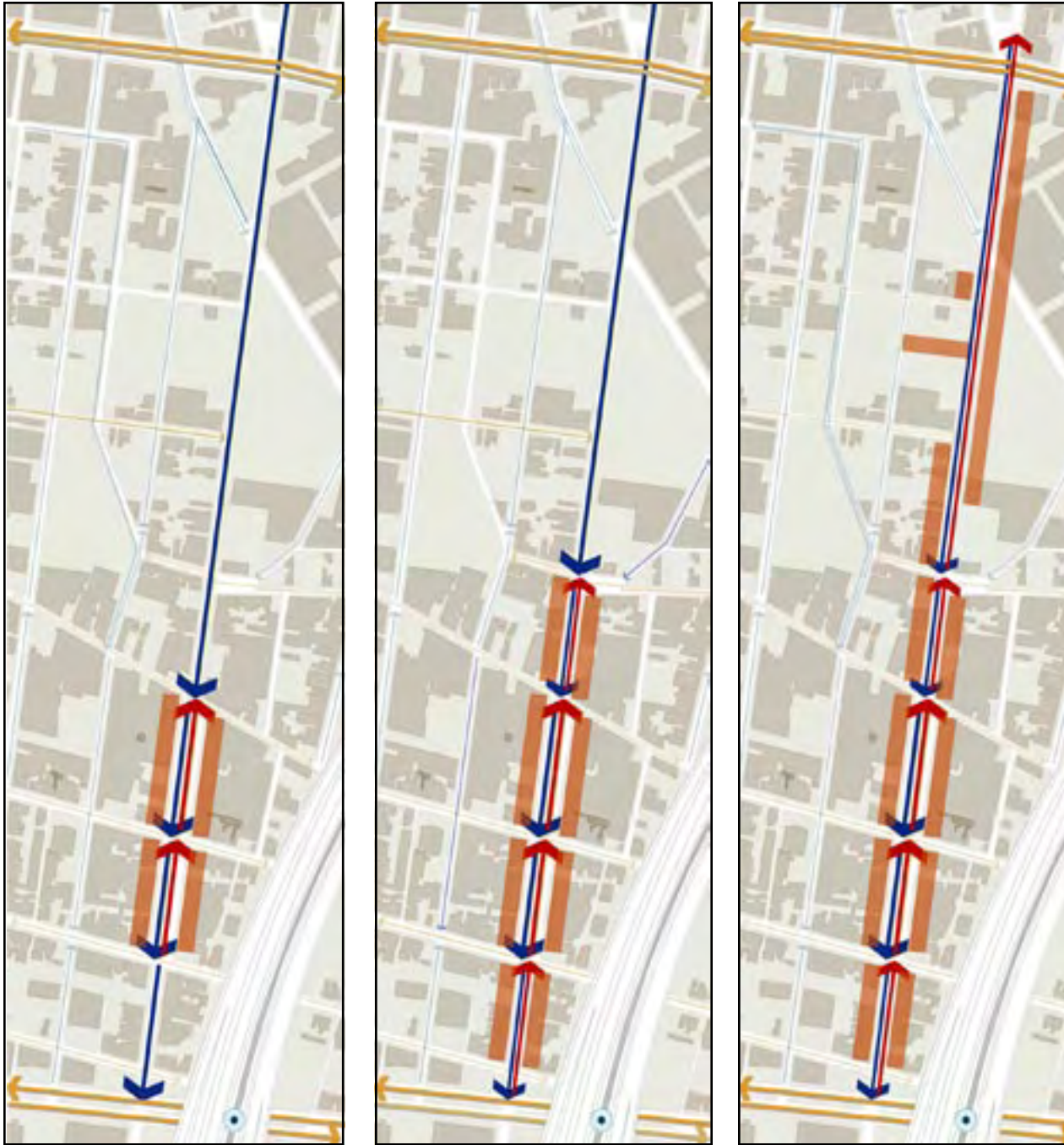
Traffic flow alternatives. Left: two-way between Fairmount & Poplar. Middle: two-way between Spring Garden & Laurel. Right: two-way between Spring Garden and Girard.
