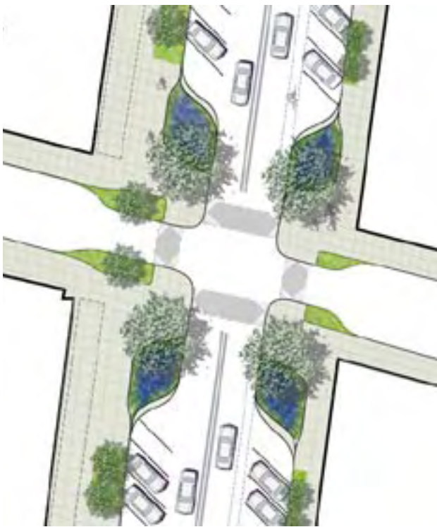
Top: Potential section of 2nd Street with a widened sidewalk. Bottom: Potential Green approach to the design of 2nd Street intersections
