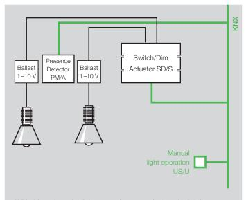
\* With this variant, the light sensor is not required as the brightness measurement and the lighting controller is integrated in the presence detector. The dimming values are sent via KNX to the Switch/Dim Actuators. In larger systems this can lead to high data transfer rates on the KNX line. Presence-dependent control is also possible for variants with DALI ballasts or with Room Controllers.
