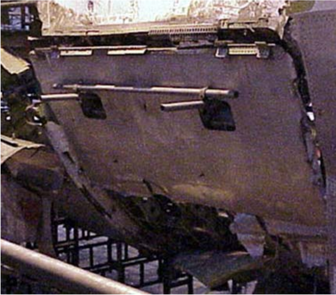
Pan Am Flight 103 Forward cargo door showing missing aft and forward pressure relief doors.
