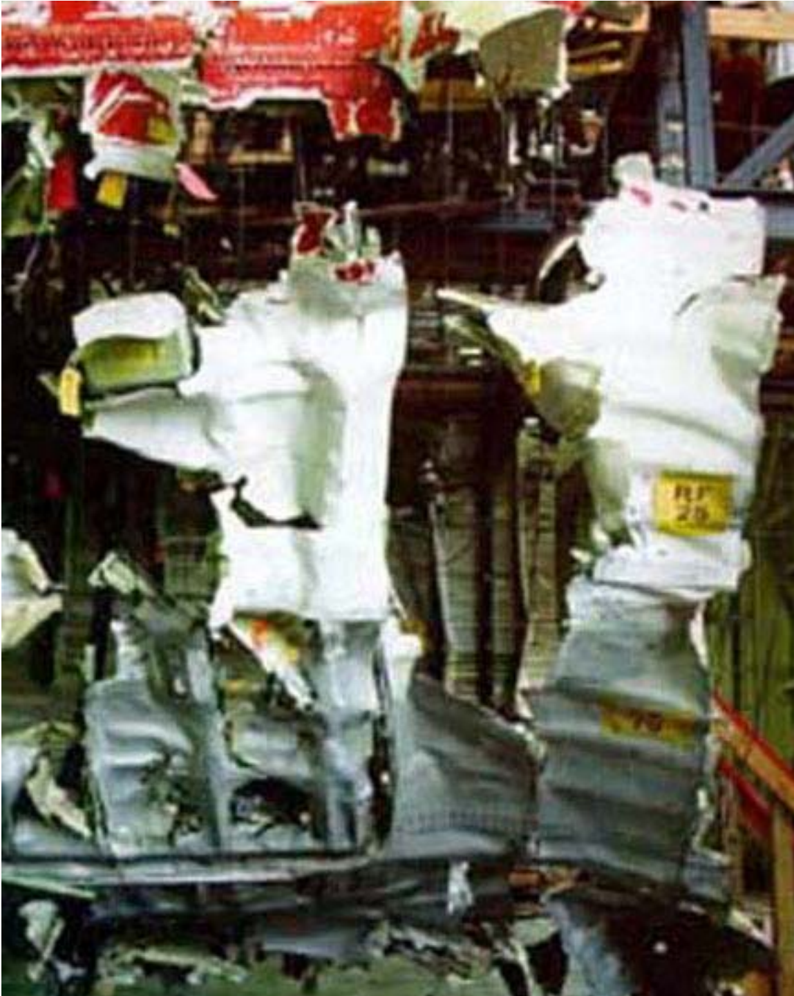
Trans World Airlines Flight 800 Forward cargo door showing separated and replaced forward pressure relief door.
