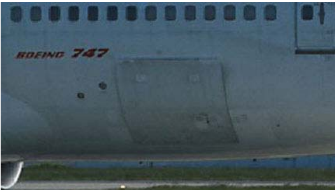
Above: Closeup of Boeing 747 closed forward cargo door showing manual locking handle, upper hinge, over pressure relief doors, passenger windows above door, and R2 door.
