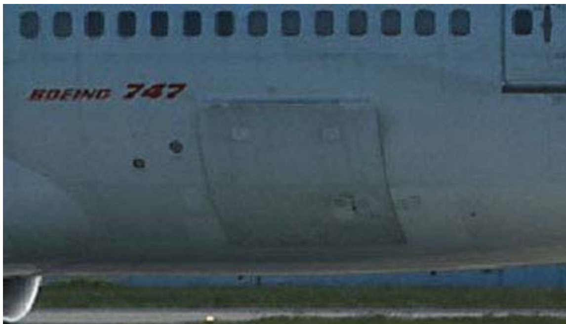
Normal Boeing 747 forward cargo door showing aft and forward pressure relief doors near top hinge.
