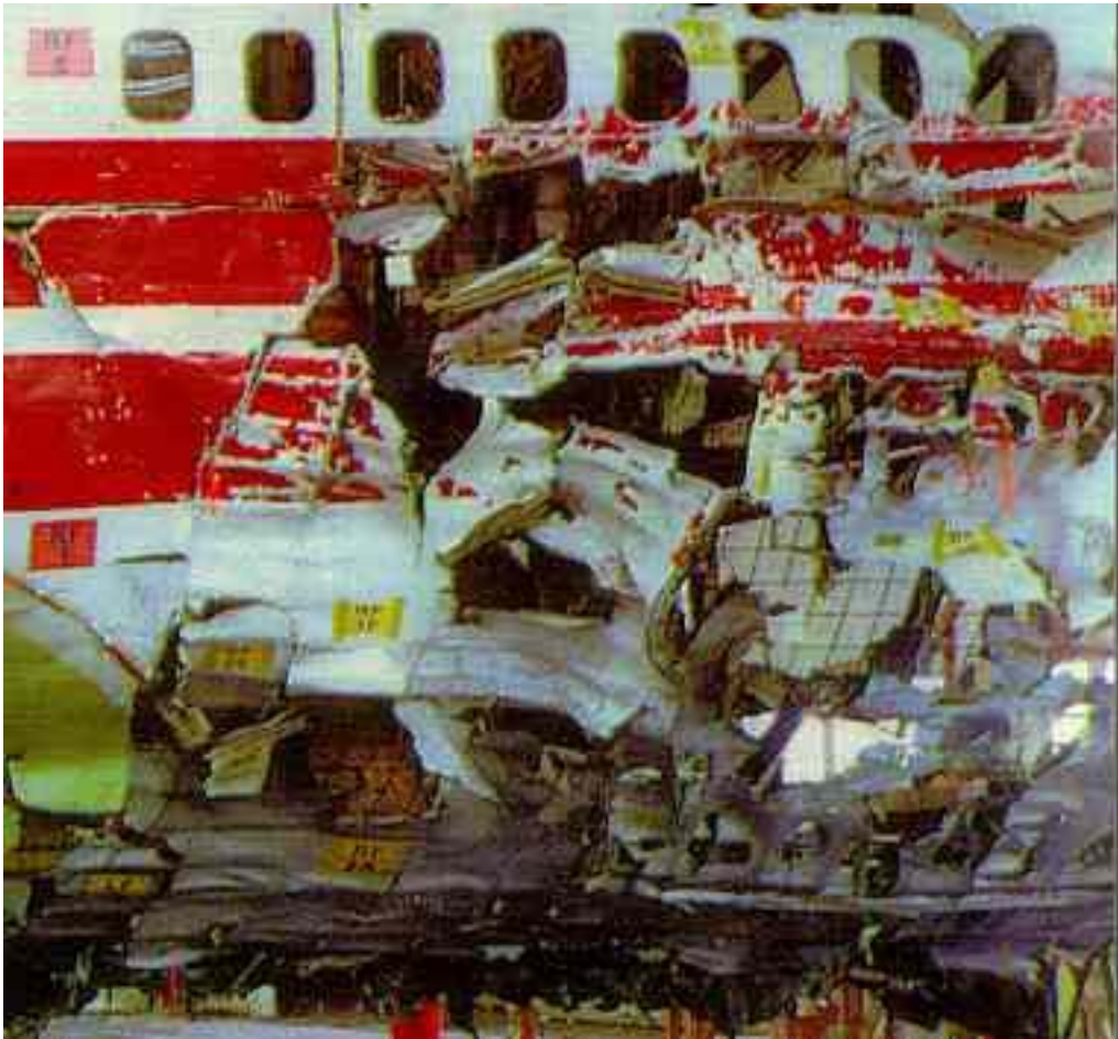
Right side of aircraft, nose to right, forward cargo door area revealing red paint smears found only in this area of Trans World Airlines Flight 800.
