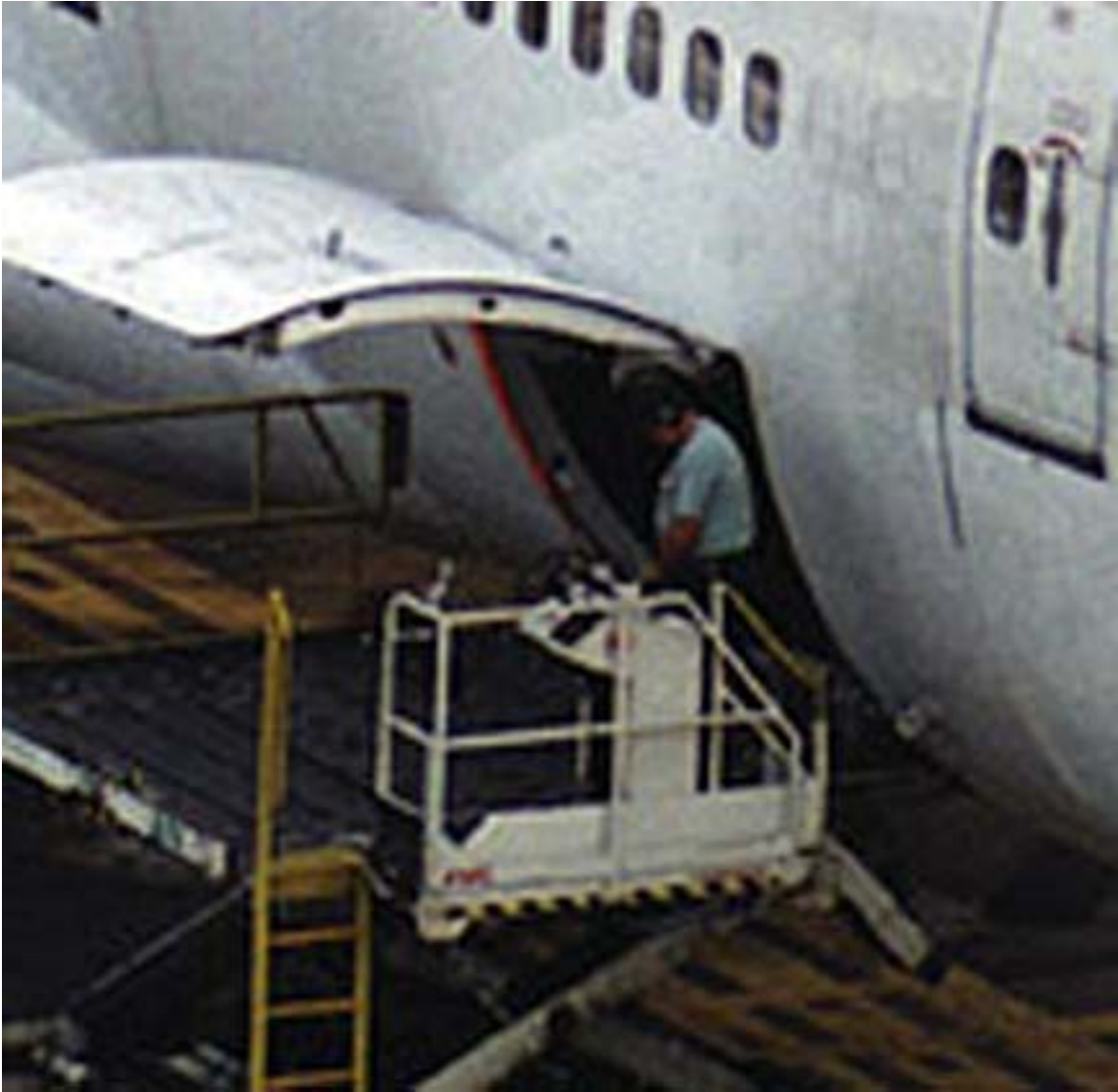
Above: Closeup of open forward cargo door showing open manual locking handle, several of the bottom eight latches, forward leading edge midspan latch, and the aft leading edge midspan latch pin.
