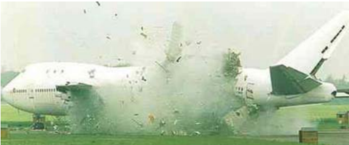
Staged bombing of a Boeing 747 at Bruntingthorpe UK showing the massive damage which occurs when a real bomb goes on in a Boeing 747.
