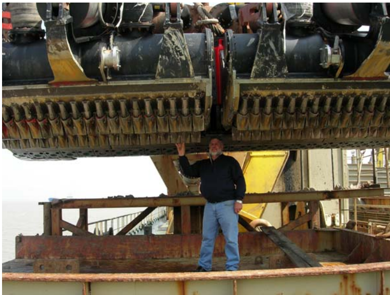
Left: AMOU Industrial Officer (VIC) Steve Groves standing under drag head of trailer-suction dredge “Fairway”
