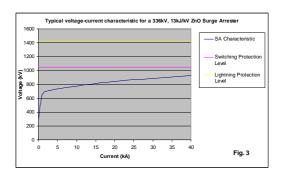
The rating of the surge arresters will have been assessed from TOV requirements and from manufacturers data a surge arrester model can be included in the system model.
