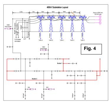
Performing various studies, representing the overhead line and substation will reveal the protective level of the arrester and from this the safety factor for this system configuration can be assessed. IEC 71
