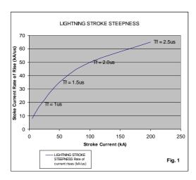
Having determined the insulation required for the line it is usual to find the lightning withstand level is in excess of commercially available lightning impulse withstand levels (LIWL) of the substation equipment. Thus, unless precautions are taken, overvoltages entering the station can cause undue insulation failure.
