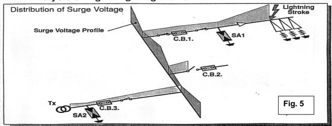
recommends a safety factor for lightning withstand of 1.25 for 550kV equipment (safety factor = LIWL / protective level). A lesser safety factor of 1.15 is normally adopted for the switching withstand level.
