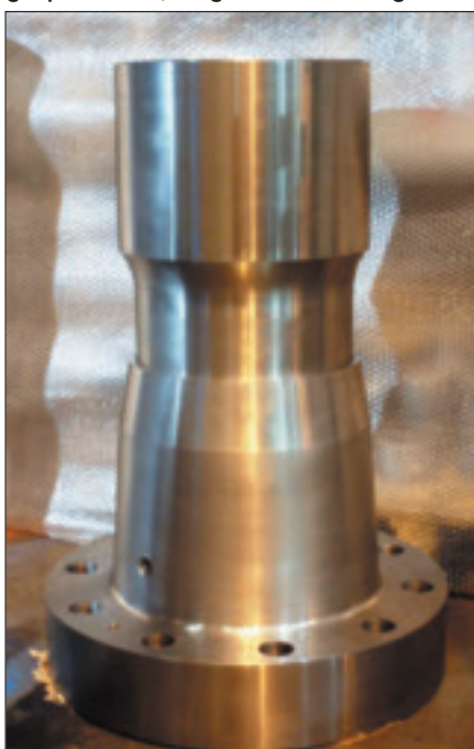
A complete shrink-fit flange produced during the development and testing programme. The short piece of main pipe is held tightly within the body of the flange.
