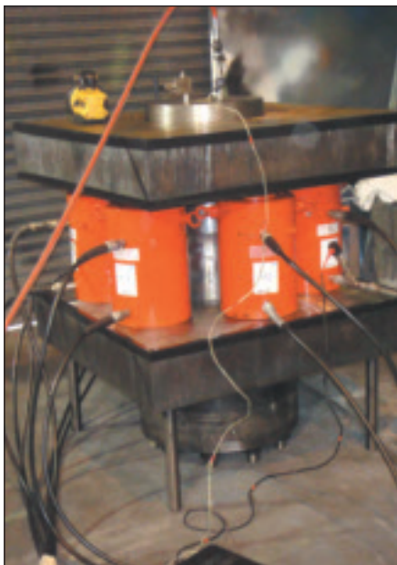
Pressure testing of completed flanges under various tension and bending loads using powerful hydraulic jacks. Some flanges were tested to destruction to see how the various sealing mechanisms performed.
