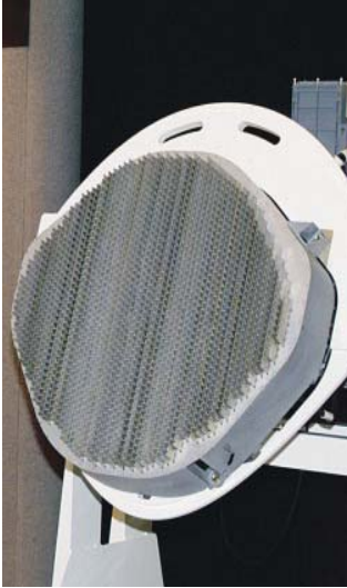
Figure 25. The AESA Antenna Used in the AN/APG-77 Radar 27
