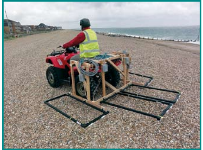
Suspended RFID Antenna Array mounted on an All Terrain Vehicle (ATV), photo courtesy of Havant Borough Council
