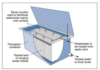
Figure 3. Schematic of textile filter for the treatment of septic tank effluent.
