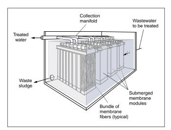
Figure 7. Schematic of a membrane bioreactor for the treatment of wastewater.
