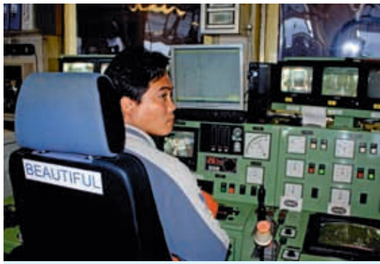
Perez Alvin is in command of the mighty winches (right). With the help of their arm-thick cables, he pulls the Castoro Sei towards the distant kedge anchors.
