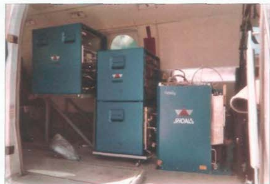
Figure 3: SHOALS-1000T as installed. The operator console is to the left, power and cooling are in the center stack, and the laser, IMU and camera are to the right.
