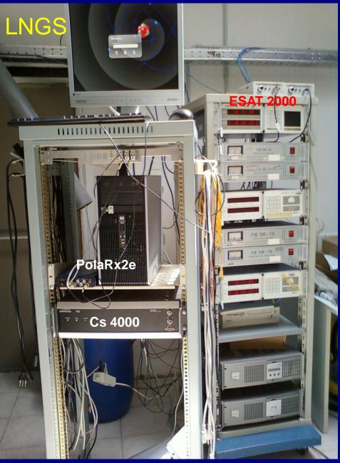
Standard GPS receivers ~100 ns accuracy: CERN Symmetricom XLi (source of General Machine Timing) LNGS: ESAT 2000
