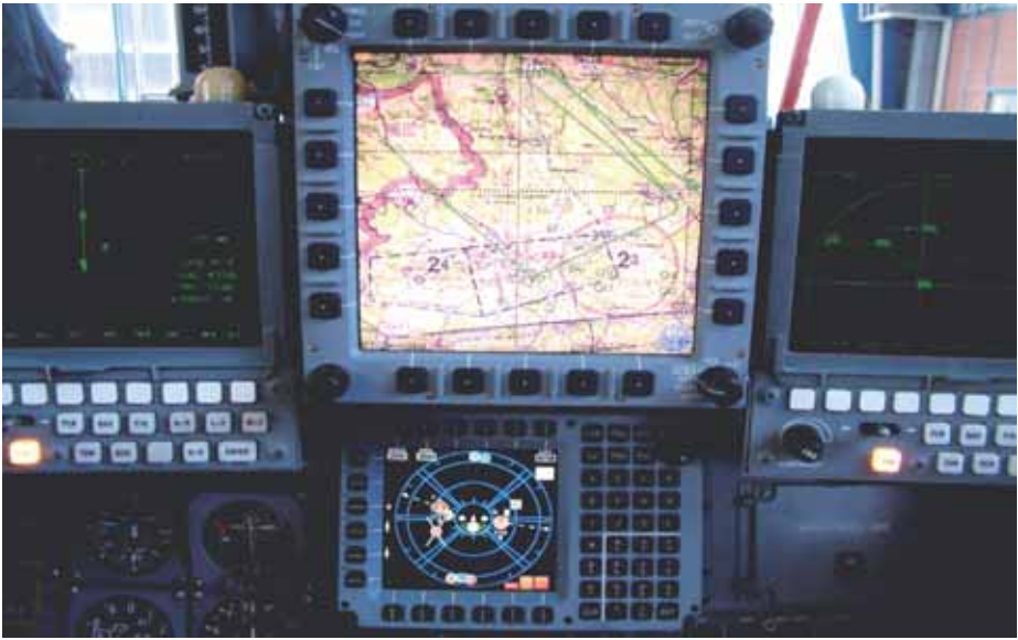
TORNADO with Navigator Head Down Display (NHDD) and Central Display Unit (CDU).
