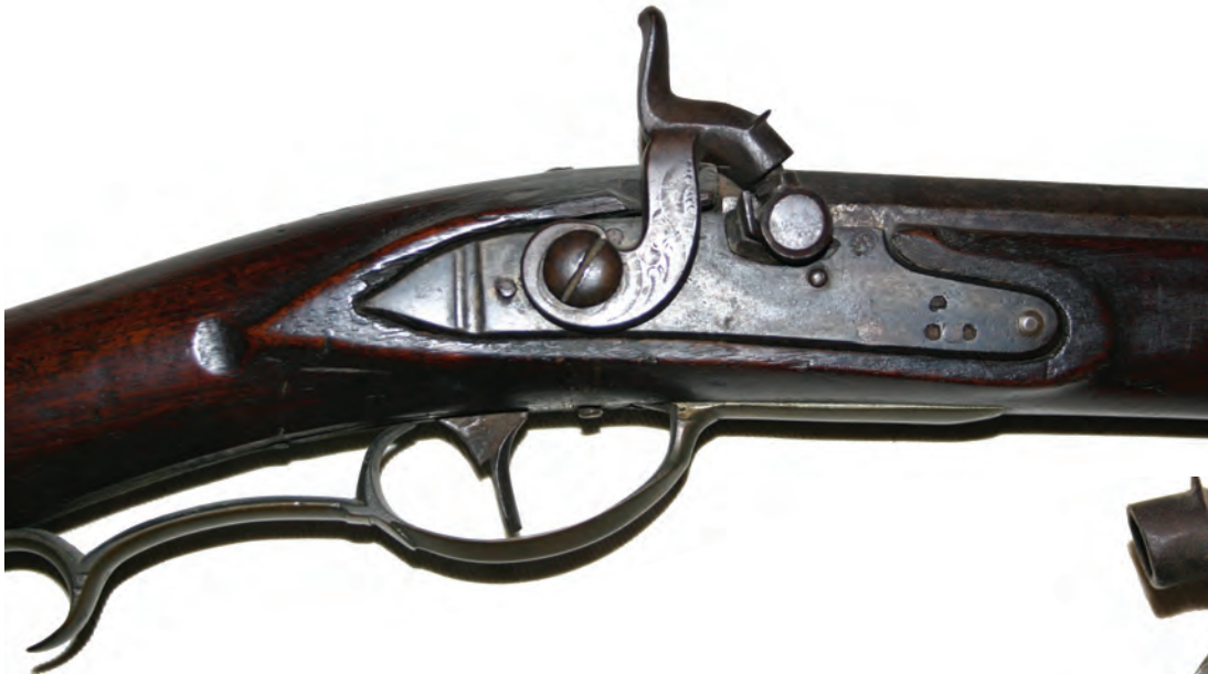
Figure 9. Lock on the P. Gonter contract rifle. A typical imported lock used on most of the 1807 contract rifles which has been converted to percussion.
