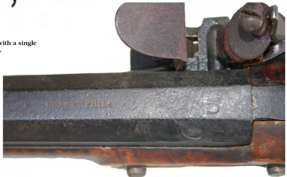
Figure 14. J. Henry's name, US mark and proof mark on barrel of 1807 contract rifle.
