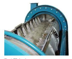
Fig. 1 TR dry cleaner – screen cage open, view of the rotor and paddle
