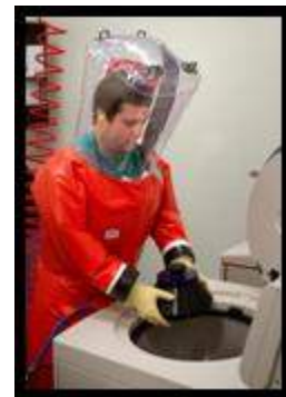
Figure 1-7. Researcher in BSL-4 PPE placing a rotor in a centrifuge.
