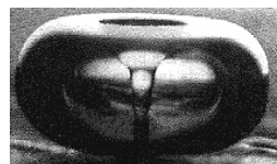
Transient bubble collapse with characteristic "jet".
