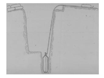
**Fig. 2-3.** A typical German chemical cylinder set up and ready for discharge. The discharge from thousands of cylinders created the gas cloud. Reprinted from Army War College. *German Methods of Offense*. Vol 1. In: *Gas Warfare*. Washington, DC: War Department; 1918: 14.
