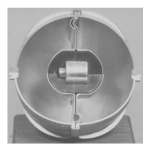
**Fig. 2-54.** The M139 4.5-in. spherical sarin bomblet used in the Little John rocket. The vanes on the outside of the bomblet created a spin that then armed the impact fuze. The explosive burster is in the center and sarin fills the two outer compartments. Photograph: Chemical and Biological Defense Command Historical Research and Response Team, Aberdeen Proving Ground, Md.
