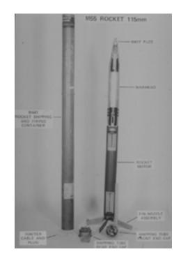
**Fig. 2-52.** The M55 115-mm rocket could hold the nerve agents VX or sarin. The problem was the aluminum warhead, which began leaking soon after production. Photograph: Chemical and Biological Defense Command Historical Research and Response Team, Aberdeen Proving Ground, Md.
