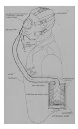
**Fig. 2-19.** A schematic diagram showing the M1 Service Gas Mask. The M1 eliminated the nose clip and mouthpiece of the box respirators of World War I vintage. By directing the incoming air over the eyepieces, it also helped eliminate lens fogging. Photograph: Chemical and Biological Defense Command Historical Research and Response Team, Aberdeen Proving Ground, Md.
