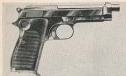
Big Beretta Brigadier 9mm pistol has cross-bolt safe, turning barrel catch.
