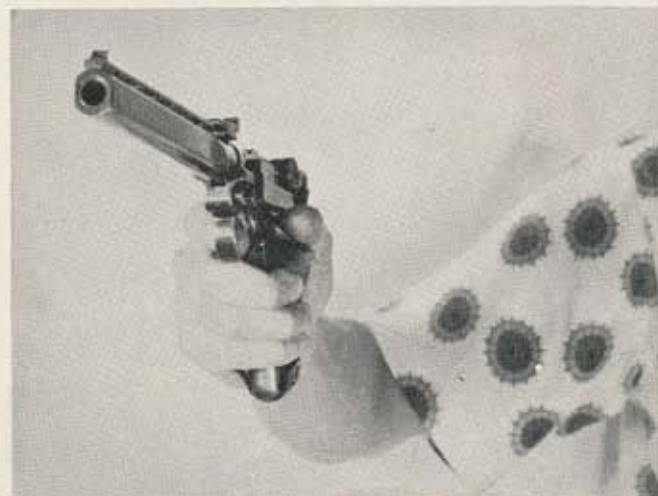
Slab-sided .45 barrel gives added mass, softens shock of big caliber recoil. Thumb-rest grips on new match pistol aid shooting. Left, shots load in fixed magazine.
