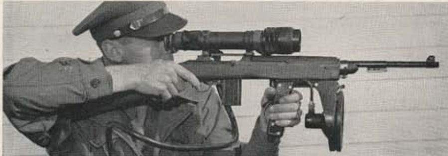
Snooper-scope has converter tube inside that changes invisible infra-red projector by stock flood light into image of target with phantom "V" sight in scope field.
