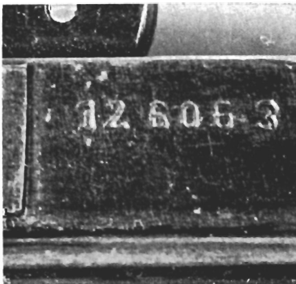
Enlargements of serial numbers in Browning imitations shows similar number stamping in some figures, suggests one single handyman may have made all pistols after one genuine Browning pistol which bore serial number of #126063.
