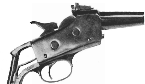
New Micro rear sight was put on breech, tangs bent and hammer spur lowered in pistol conversion.
