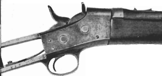
Remington receiver tangs must be bent and spring altered for large-size custom grips to take up kick.
