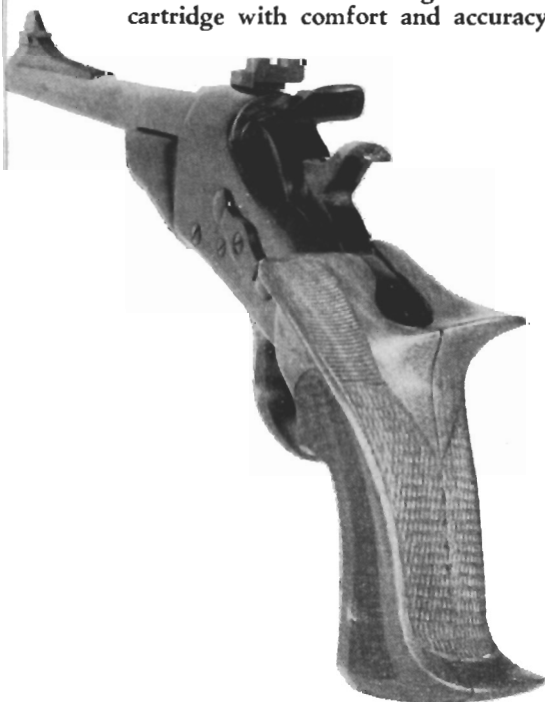
Special form-fitting grips made by Steve Herrett allow firing .257 rifle cartridge with comfort and accuracy.
