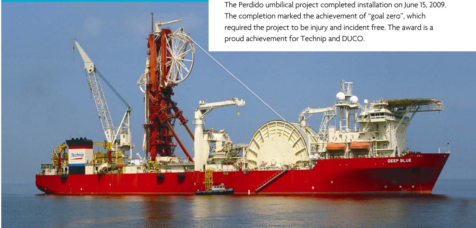
Technip used its high-technology Deep Blue vessel to lay pipelines and risers for the Shell Perdido project
