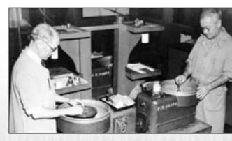
Optical glass blanks being shaped for preparing lenses and prisms, c.1947.
