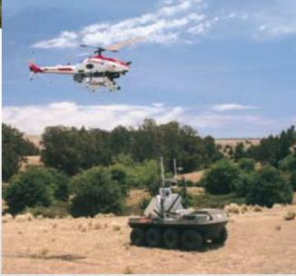
Working with the universities of Sydney and Adelaide, DSTO demonstrated the ability of an umanned ground vehicle to operate autonomously in difficult terrain by downloading maps from an unmanned aerial vehicle.
