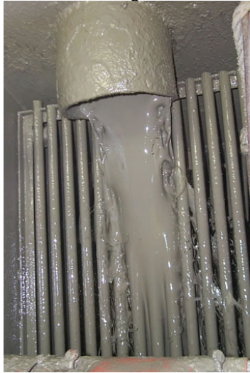
Figure 2: Drilling mud exiting flowline
