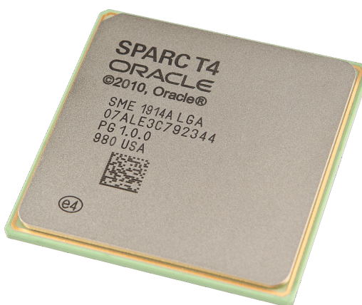
Figure 1. The SPARC T4 processor features 8 cores and 64 threads with 5x the single thread performance of the previous generation
