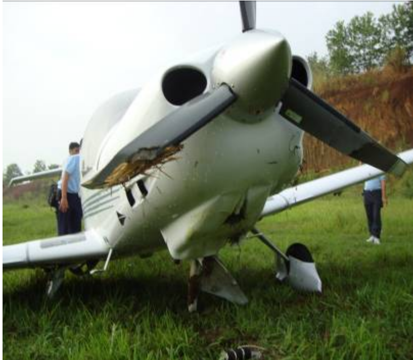
Figure 3: Damaged nose and right main landing gear, and propeller blades
