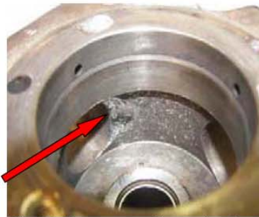
Pic. 32: Damage marks at chamber E
