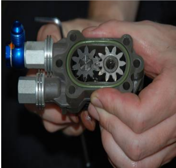
Figure 7: Feed Pump/ Low Pressure
