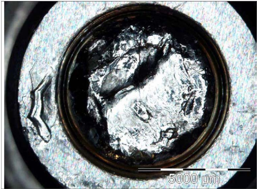
Pic. 48: Fracture surface of the piston, which is still seated inside the cylinder.
