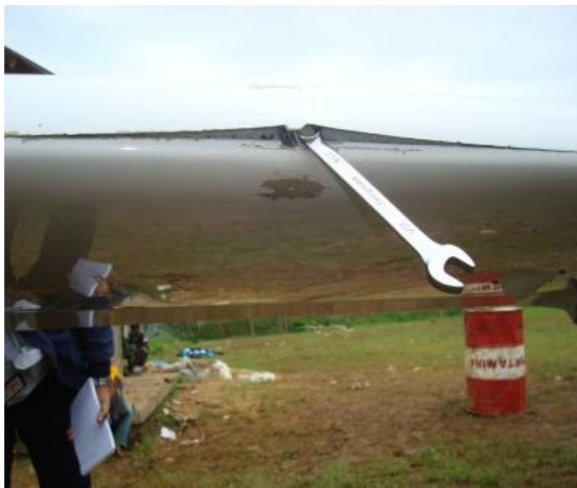
Figure 4: Right wing leading edge split in 2 locations
