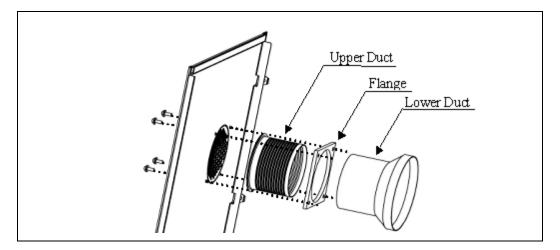
Figure 3. Chassis Air Guide Exploded View With Screws
