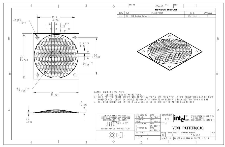
Figure 10. Vent Pattern, Chassis Air Guide
