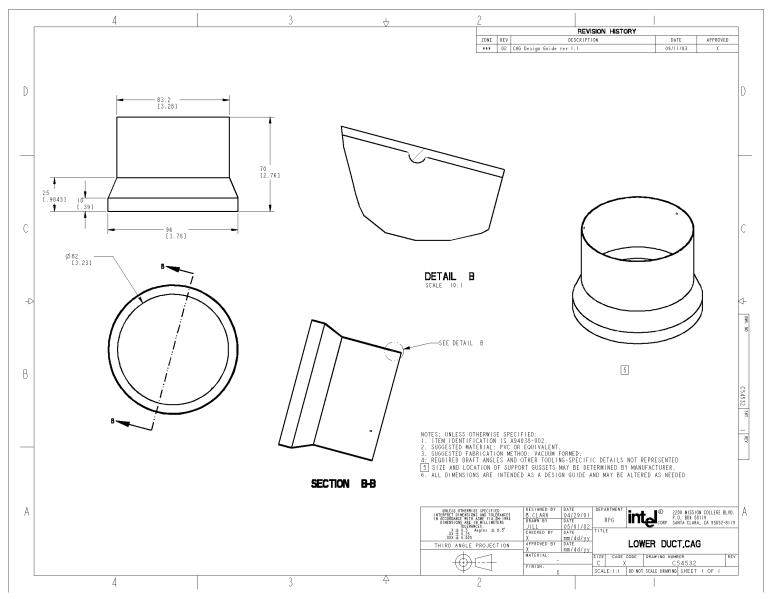
Figure 8. Lower Duct, Chassis Air Guide
