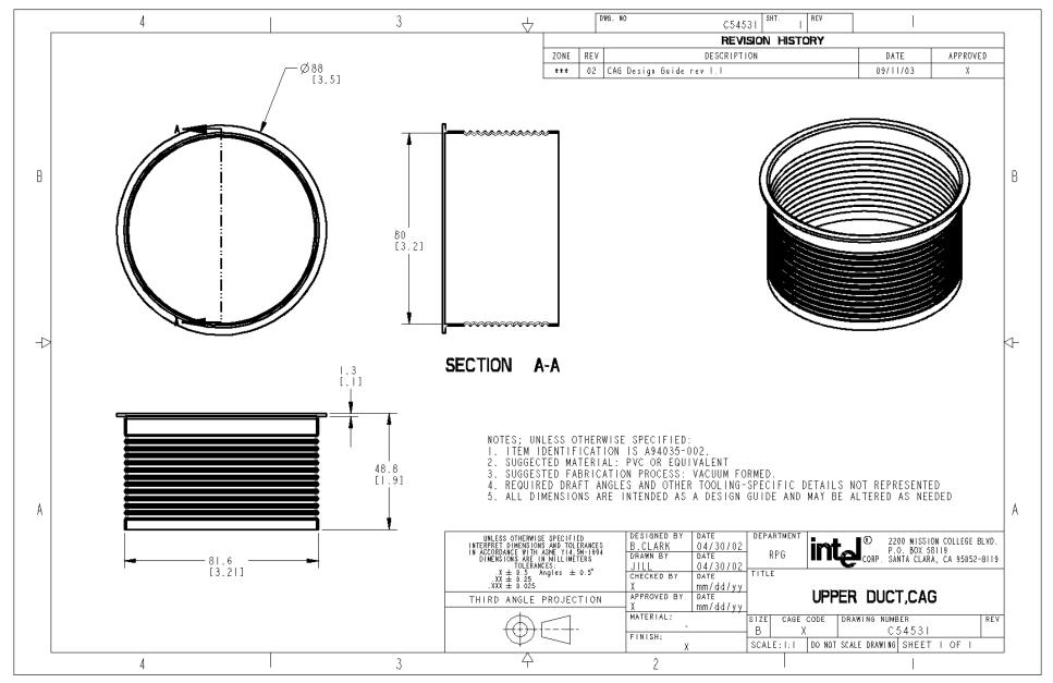
Figure 7. Upper Duct, Chassis Air Guide
