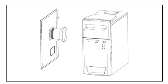
Figure 1. Typical Tower Platform With Chassis Air Guide
