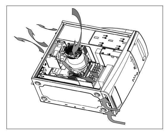
Figure 2. Chassis Air Guide Typical Airflow Pattern
