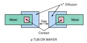
Fig. 3 — Although the lateral interconnection circuit has a relatively high resistance associated with it ( $\approx 100 \Omega$ ), it requires no nonstandard fabrication steps and can be produced with conventional CMOS technology.
