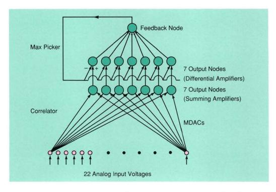
Fig. 8 — This neural net consists of 154 MDACs connected to seven summing amplifiers. The outputs of the summing amplifiers are connected to seven differential amplifiers. The differential amplifiers and the feedback node comprise a max-picker circuit that finds the vector registering the strongest correlation with the input vector.
