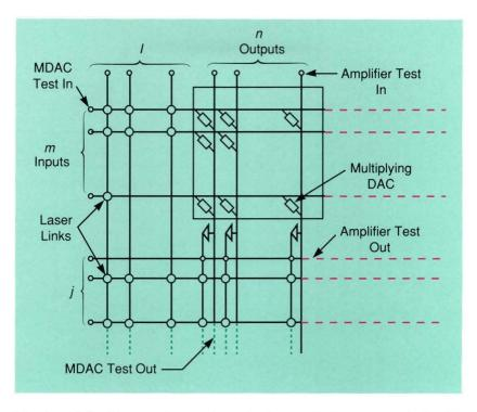
Fig. A — A flexible neural-network application can be implemented with this restructurable VLSI array of mutiplying digital-to-analog converters (MDAC), summing amplifiers, and laser links.
