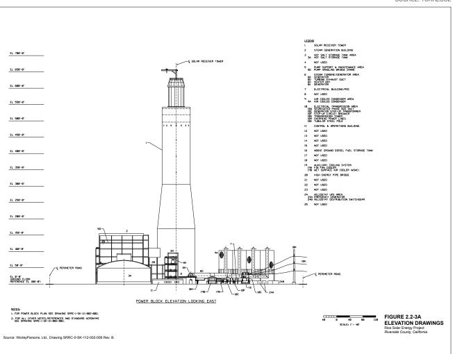
Drawings of a SolarReserve Solar 150 MW tower to be installed in Rice County CA®
