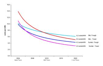
The red curve on the chart above represents the Sargent & Lundy cost projection for towers, while the mauve curve represents the SunLab tower projection. The main difference between the two projections is the cumulative installed capacity assumed by each. In the original report, these were referenced to an installation timeline from 2004–2020, but the more important factor in achieving the cost reductions was not the timeline but the total installed capacity.
