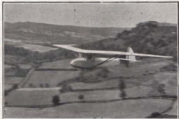
FALCON III. —A two-seater sailplane with side-by-side seating; produced by Slingsby Sailplanes. Span, 58 ft.; area, 286 sq. ft.; weight, 500 lbs. The "Daily Dispatch" has presented the Derbyshire and Lancashire Gliding Club with a machine of this type, which recently attended the International Gliding Contest in Germany and there set up an international duration record for two-seater sailplanes.
