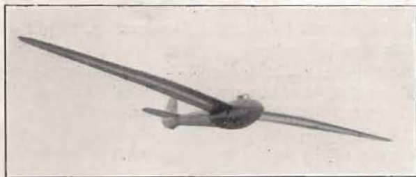
RHÖNSPERBER. —A successful German design by Hans Jacobs of Darmstadt; first appeared in 1935. Span, 54 ft. 4 ins.; wing loading, 3.1 lbs. per sq. ft.
