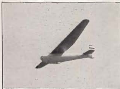
RHÖNBUSSARD. —An earlier design by Hans Jacobs. Span, 47 ft.; wing loading, 3.1 lbs. per sq. ft.
