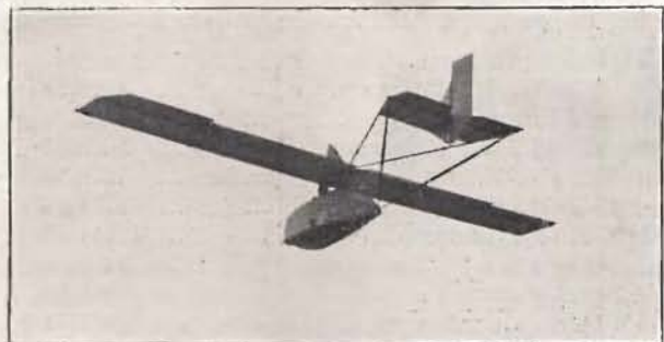
SECONDARY SAILPLANE. —Several types of machine used for training pupils in soaring flight may be seen at this meeting, such as the "Falcon I" and "Kadet." The one shown above is a Dagnall primary training machine with a cockpit added; it may be used for "spot landing" competitions on days unsuitable for soaring.
