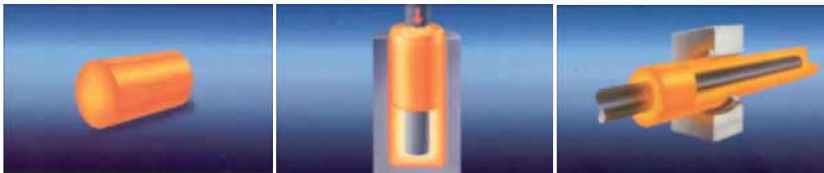
Figure 4.2.6 Lingot - Perçage – Etirage
