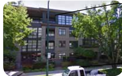
The 4th floor is expressed with darker materials, a floor level cornice line and a larger, divided glazing pattern.
